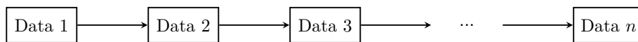
Figure 1.4.: Singly Linked List Structure. A singly linked list consists of a sequence of elements, where each element points to the next element in the sequence.
